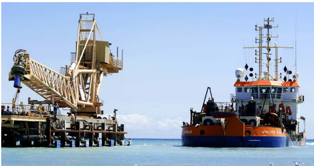
Cockburn cement's new trailer suction dredge 'Volvox Anglia' in operation at Woodman point.
