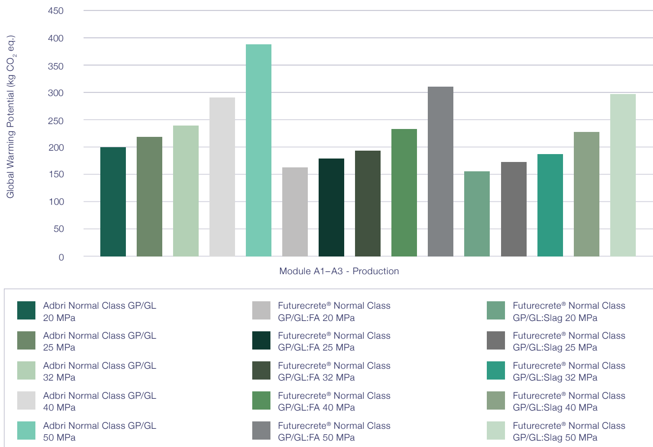
Figure 3 | Contributors to GWPT impacts of Adbri Normal, Futurecrete® and Futurecrete® Ultra Class Concrete in the different life cycle stages
